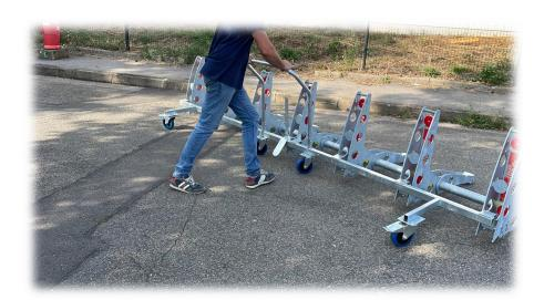
To remove the trolley, start by undoing the lock by pressing the handle and the pedal, then tilt the trolley forward to remove the module hooks.
