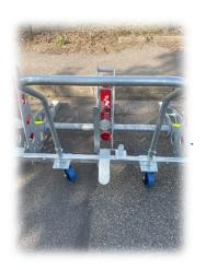
Tilt the lock vertically behind the central module
